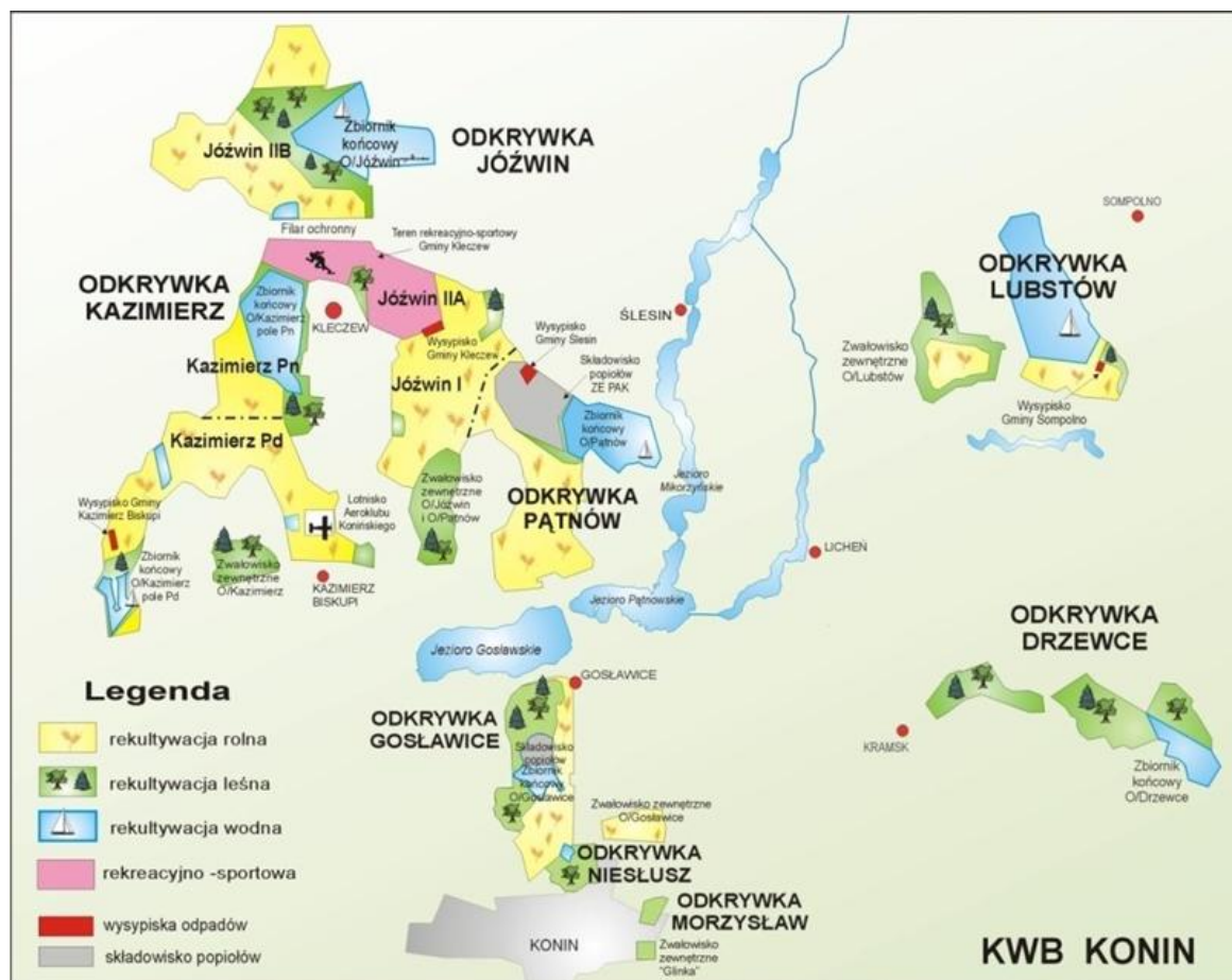
Figure 58 Reclamation of mining sites in the Konin Lignite Mine. Source: Kasztelewicz et al., 2010.
