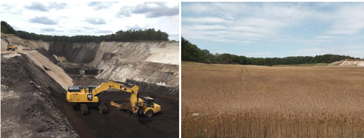
Figures 12-13. Mining area in August 2020 with active mining operations (left). The same post-mining area in November 2022 reclaimed in agricultural direction (right).
